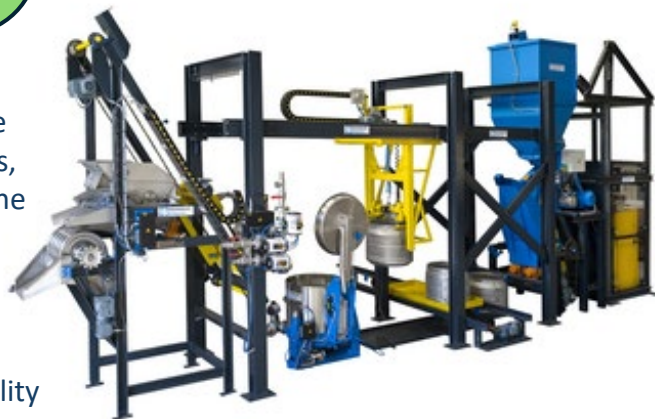
Plastics recycling line with automated Model SA Filtering Centrifuge
